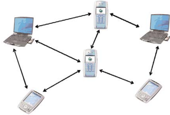
MobileMAN: two users manage to communicate with each other also in the absence of a direct connection. No fixed infrastructure, no central authority.
