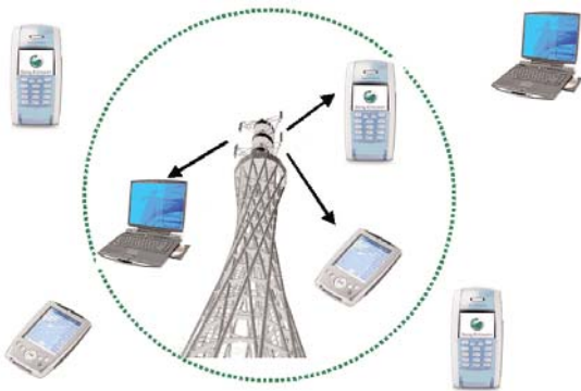
Traditional mobile network: the central node (aerial) connects the wireless nodes; nodes that are too far away cannot communicate.
